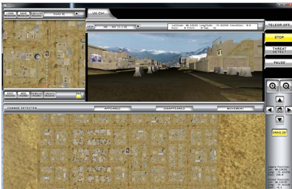
The vehicle will move along the route until it reaches the end point. Edit Route, Add Point, Remove Point, and (detailed later in the document) Create Route can be used in the same manner as in the editor, as long as the buttons are enabled.
