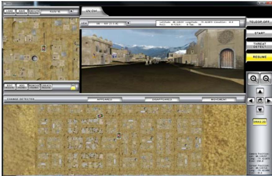
This is a standard layout of an OCU, mainly intended for simple observation of a single vehicle taking a route and the environment around it.
